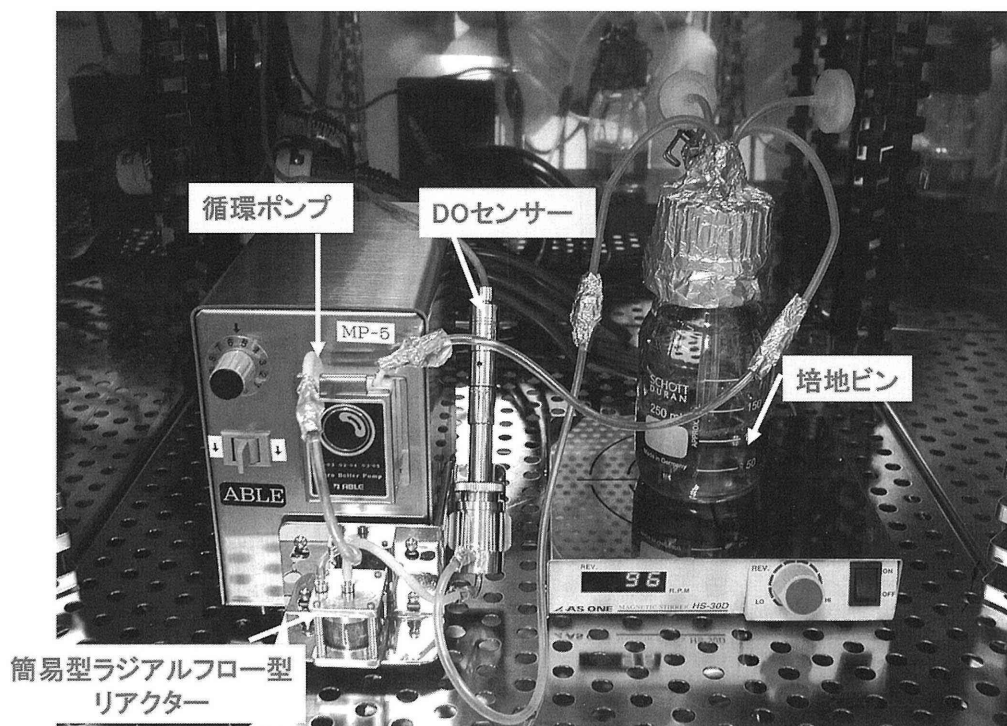
Fig. 2 Overview of the small RFB System
